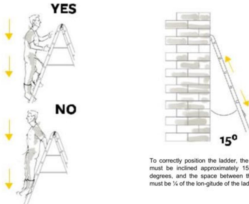
To correctly position the ladder, the ladder must be inclined approximately 15 to 20 degrees, and the space between the wall must be  $\frac{1}{4}$  of the longitudinal of the ladder.
